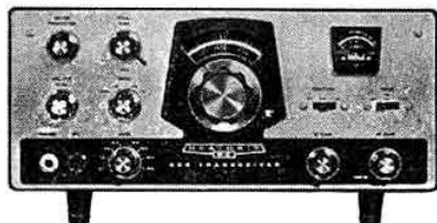
HW-100 5 Band SSB-CW Transceiver . . . Solid-State (FET) VFO covers 80-10 metre bands. Switch selector USB LSB or CW. 180 watts input PEP SSB, 170 watts input C.W. Crystal filter. Kit HW/100 18lbs £132 P. & P. 11/-
