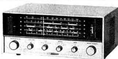
GR-64 4 Band Shortwave Receiver . . . 4 bands—3 shortwave bands cover 1 MHz to 30 MHz plus 550 kHz to 1620 kHz. AM broadcast band. Variable BFO control for code and SSB transmissions. Built-in AM antenna. Kit K/GR-64 £22.8.0 P.P. 9/-.
